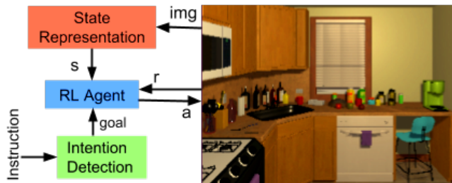
Fig. 2. The modular approach using intention detection and reinforcement learning trained for each objective to generate the sequence of actions [9].
